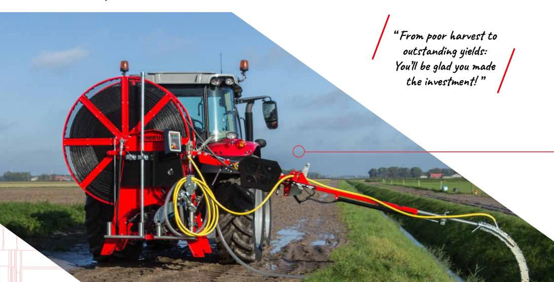
The Delta offers more ease of use as a draincleaner than the Blizz. This is the ideal machine for anyone who maintains drainage systems on a frequent basis and needs to cover a large area. This is because it offers hydraulically operated height adjustment, extension, retraction and folding of the drainage arm and length adjustment of the guide arm.
