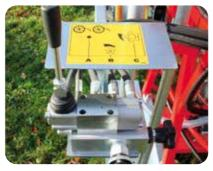
The machine comes standard with a hydraulic drive control system operated with a lever.
