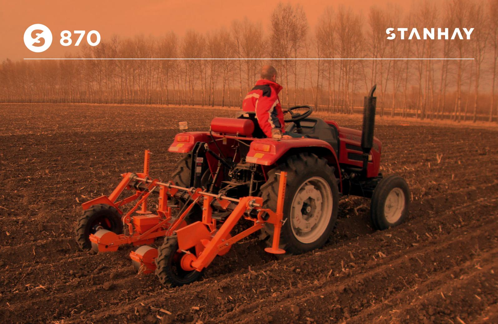
Used all over the world the 870 is the market leading belt planter. With a 7 speed pulley drive courtesy of adjustable height landwheels, the 870 can work on the flat or bed setups. Available from 2 rows up to 18 rows and capable of multiline planting, the 870 is robust, scalable and adaptable for every seed type.
