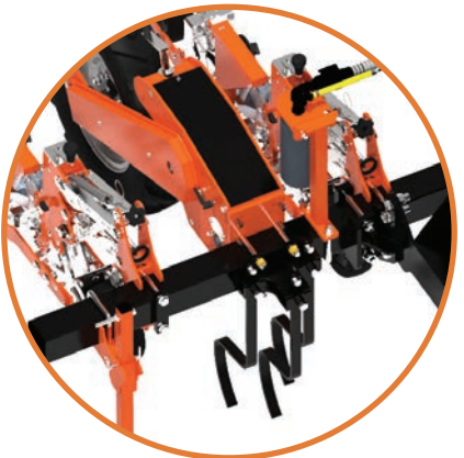
TRACK ERADICATOR TINES Track eradicator tines can be fitted to remove tractor wheel marks prior to the drill. 1, 2 or 3 tines can be fitted which are adjustable in height and available with a chisel point or A-share. They can easily be fixed out of work when not required.
