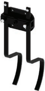
TRACK ERADICATOR TINES Track eradicator tines can be fitted to remove tractor wheel marks prior to the drill. 1, 2 or 3 tines can be fitted which are adjustable in height and available with a chisel point or A-share. They can easily be fixed out of work when not required.
